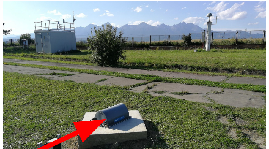
B.) Active: radar transponder
