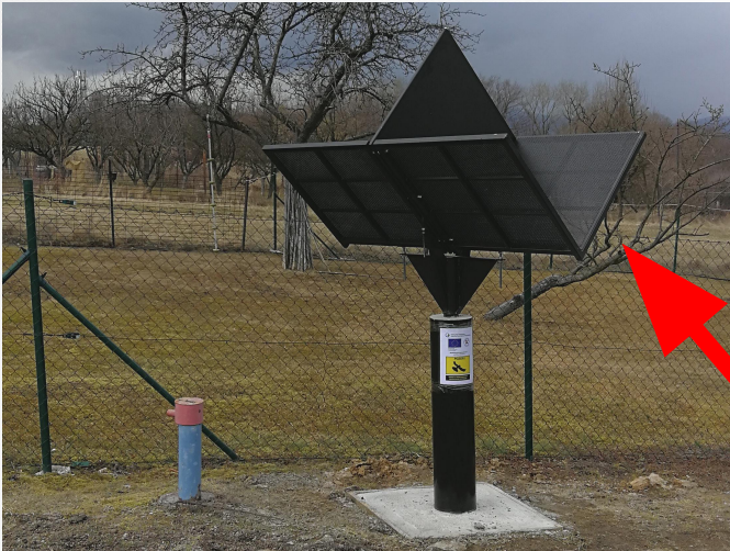
A.) Passive: corner reflector
