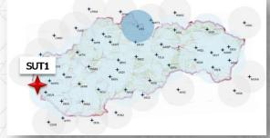
RTKNAVI connects to SKPOS<sup>®</sup> and simulates the rover standing on GKU4. The baselines composed of VRS (generated for GKU4 coordinates) and SUT1 station and GKU4 and SUT1 are computed and compared.
