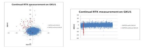
Fig.3 Results from continual RTK measurement on GKU1 marker.
